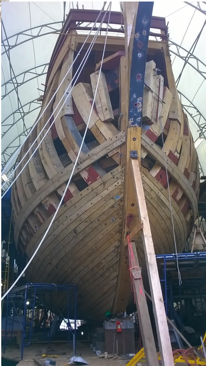
Bow of the Mayflower II with nearly all new futtocks and planking.
